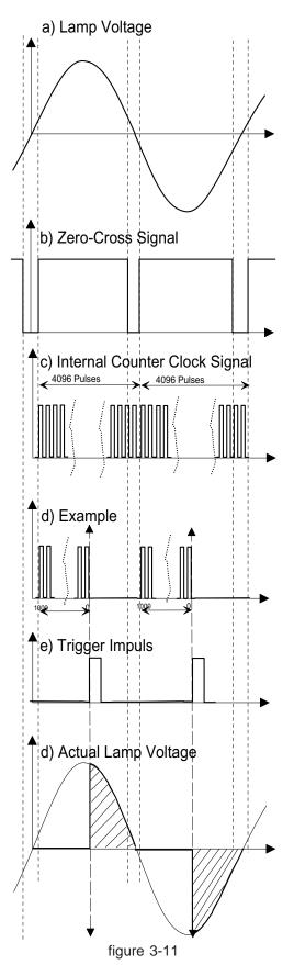
The zero-cross circuit creates an impulse whenever the LAMP voltage crosses the zero line (LAMP voltage close to zero). See figure b.
